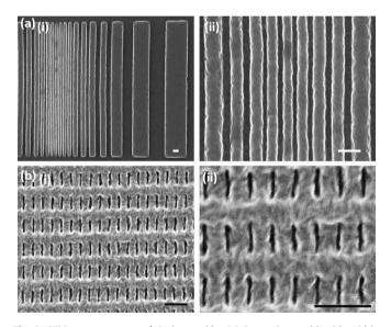
**Fig. 3.** SEM measurements of Surlyn molds: (a) Protrusion mold with widths varying from 1  $\mu$ m to sub-100 nm, (i) survey, (ii) zoom on smallest structures, (b) cavity mold with sub-50 nm structures (i) survey, (ii) zoom; scale bars correspond to 200 nm.
