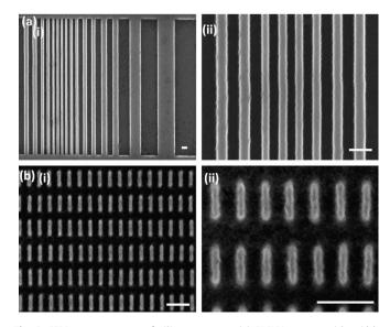
**Fig. 2.** SEM measurements of silicon masters: (a) PMMA-master with widths varying from 1  $\mu$ m to sub-100 nm, (i) survey, (ii) zoom on smallest structures, (b) HSQ-master with sub-50 nm structures (i) survey, (ii) zoom; scale bars correspond to 200 nm.
