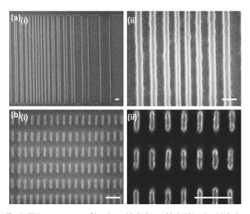
**Fig. 4.** SEM measurements of imprints with Surlyn molds in UV resist: (a) Cavity imprint with widths varying from 1  $\mu$ m to sub-100 nm, (i) survey, (ii) zoom on smallest structures, (b) protrusion imprint with sub-50 nm structures, (i) survey, (ii) zoom; scale bars correspond to 200 nm.
