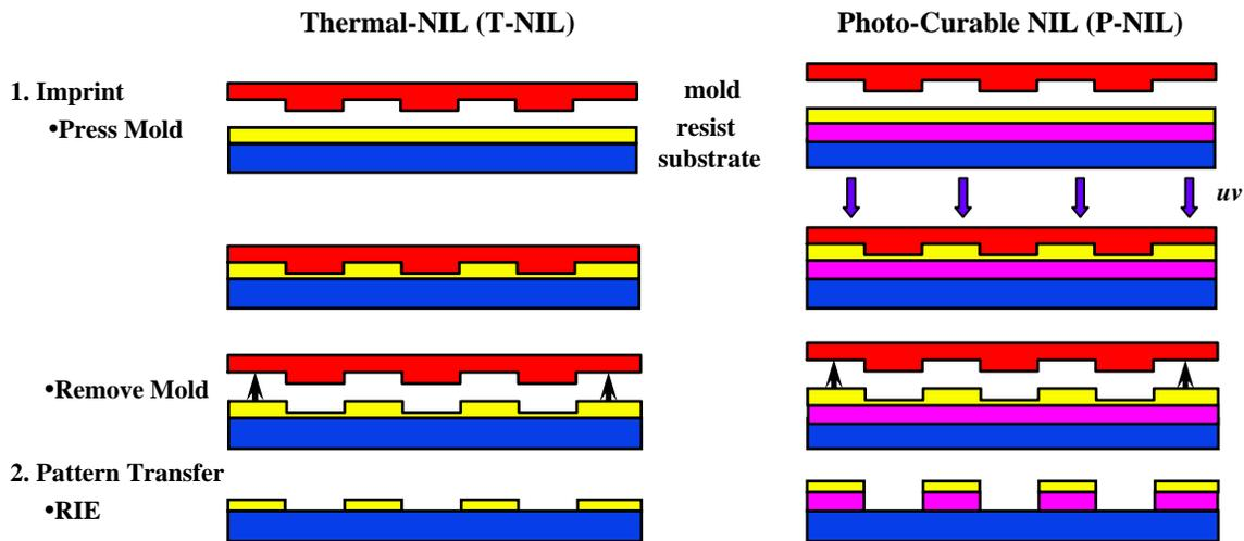
Figure 1. Nanoimprint lithography (NIL) has two alternatives, thermal NIL (T-NIL) and photo-curable NIL (P-NIL).
