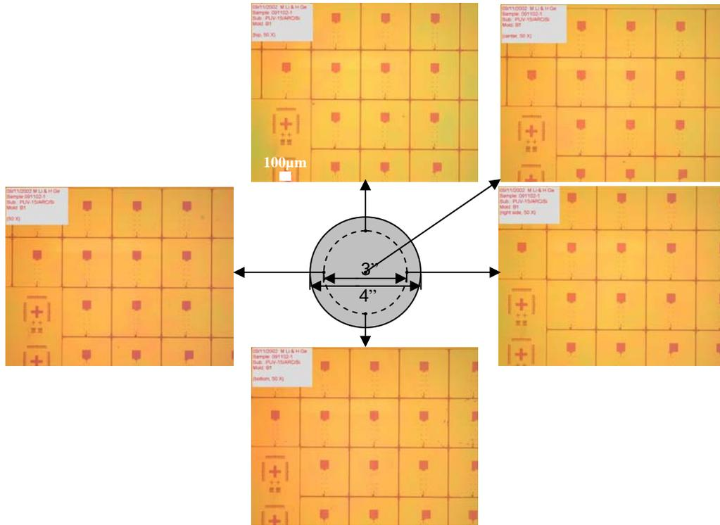
Figure 5. The gate level of MESFET circuit is imprinted in NXR-2010 over 4-inch wafer using P-NIL on NX-2000 nanoimprinter. The CD on the circuit is 1.5µm.
