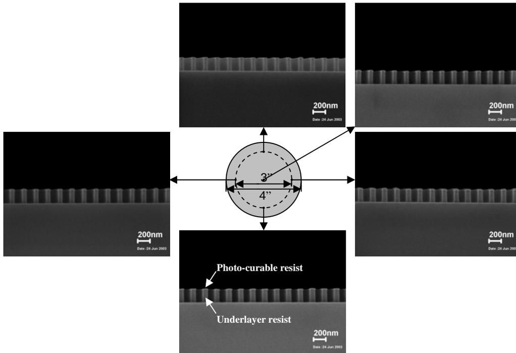
Figure 4. 200nm pitch grating imprinted in NXR-2010/NXR-3010 resist over 4-inch wafer using P-NIL on NX-2000 nanoimprinter.
