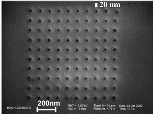
Figure 2. 100nm pitch, 20nm holes imprinted in NXR-3010 resist using P-NIL on NX-2000 nanoimprinter.
