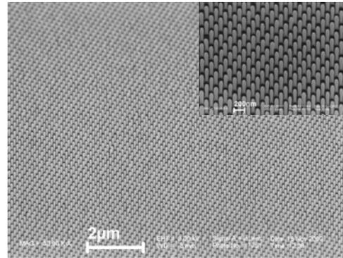
Figure 3. 200nm pitch, 65nm pillars imprinted in NXR-2010/NXR-3010 resist over 4-inch wafer using P-NIL on NX-2000 nanoimprinter.
